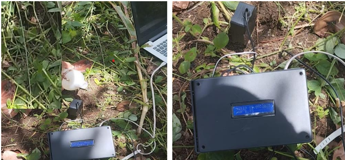
Figure 5. Watering to Check Soil Humidity and PH Tanah
